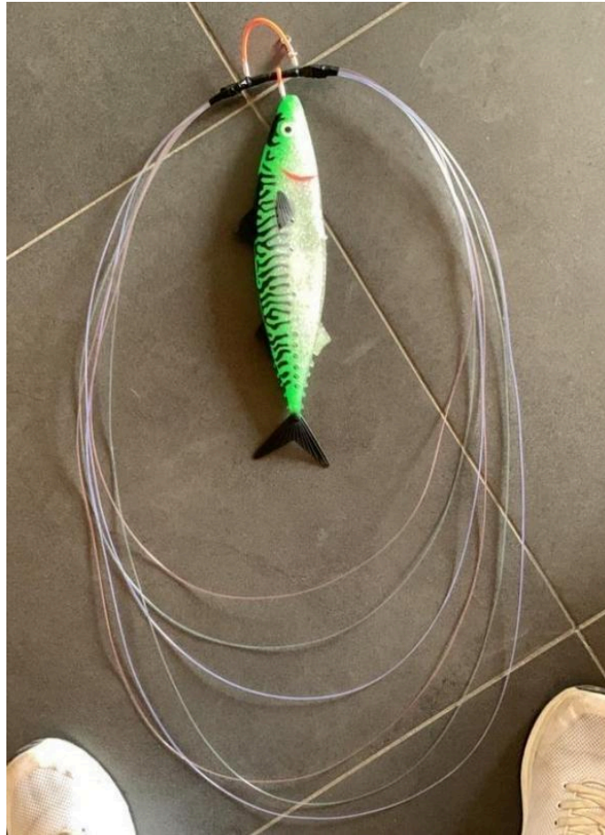
Figure 2. Trapline with mackerel lure, adapted from Garibaldi et al. 2024. The new fishing gear consists of concentric loops made up of nylon thread in different thickness and a central lure which can either be a mackerel or squid shape. Initially, fishers supplemented the lure with sardine bait and/or lights but later found the gear also works well without either.
